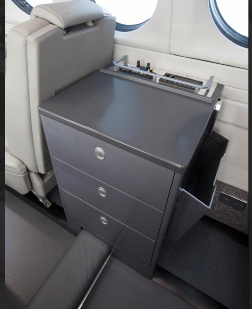
Storage cabinet with integrated communication system.
