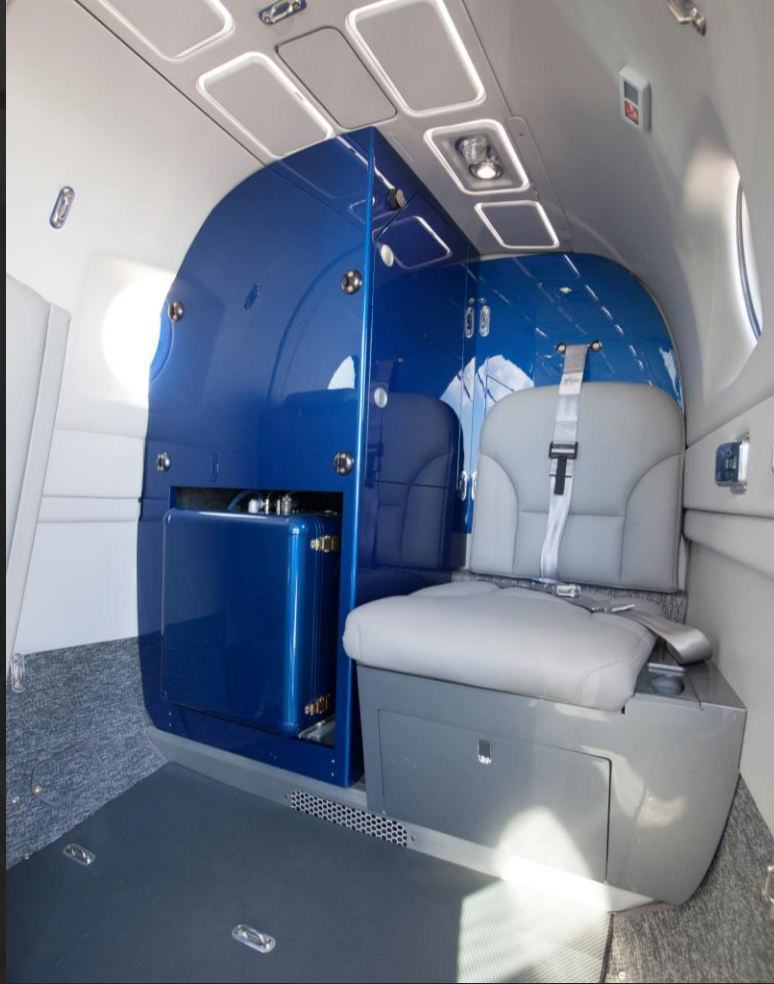
AFT supply cabinet with 10ltr LOX system and lockable storage space.
